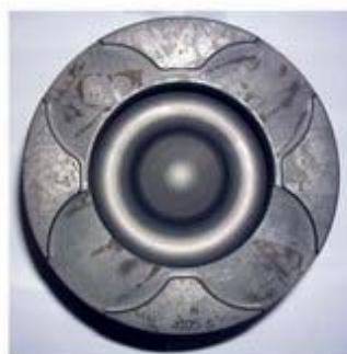
S6D140 6212-31-2151 Total Height 125.2mm, Combustion Chamber 78mm
