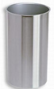
Before the liner is installed, the locating bore in the cylinder block must be cleaned carefully, and must be checked to ensure the accuracy of the dimensions and to determine whether any distortion has occurred. Out-of-center or damaged bores can be reworked for the installation of oversize liners. It is important for this that the locating bore is cylindrical, as this is what determines the geometrical shape of the inside of the pressed-in, thin-walled liner.
